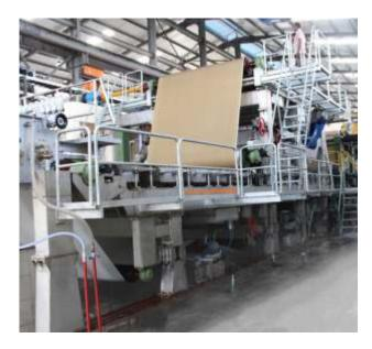
Scan Machineries engineers, designs and manufactures complete Kraft and Board Paper Machines to produce Kraft Paper, Test Liner, Uncoated and Coated Board of higher grammage (GSM). Our Paper machines have paper deckle widths up to 6m and are capable of producing paper at high speeds maintaining excellent sheet formation and quality
